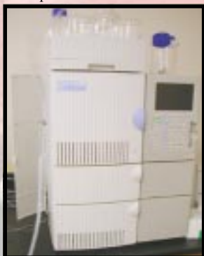
Analysis of the amino acids in wheat flour using High Performance Liquid Chromatography (HPLC).
